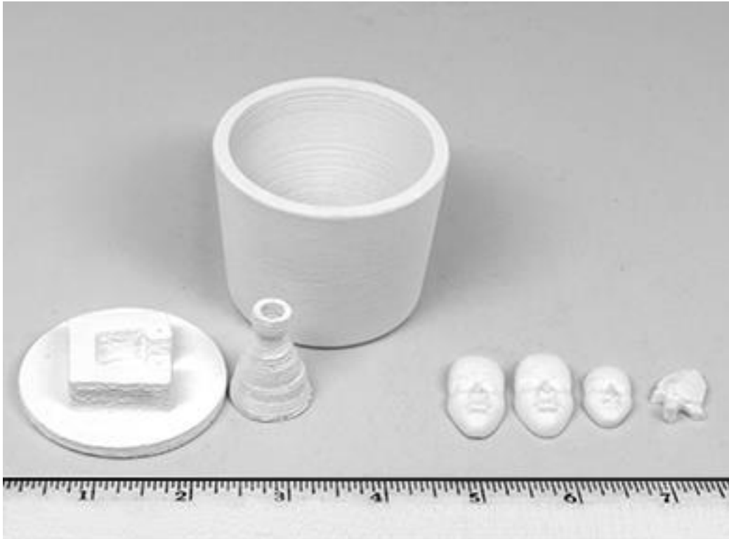
Figure 1. 3D printed parts (left) and press-formed pieces (right) after sintering at 1400°C for two hours.
