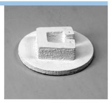
Printed ZRP part made by sintering two 3-D printed parts at 1400 C for two hours in air and then gluing them together and bonding/firing in air to 950 C for 30 minutes. Fired ZRP parts have excellent thermal shock resistance.
